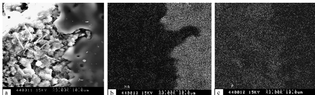
Fig. 2. SEM pictures of the OK44 specimen: (a) cement matrix, (b) distribution of Na, and (c) distribution of P.
